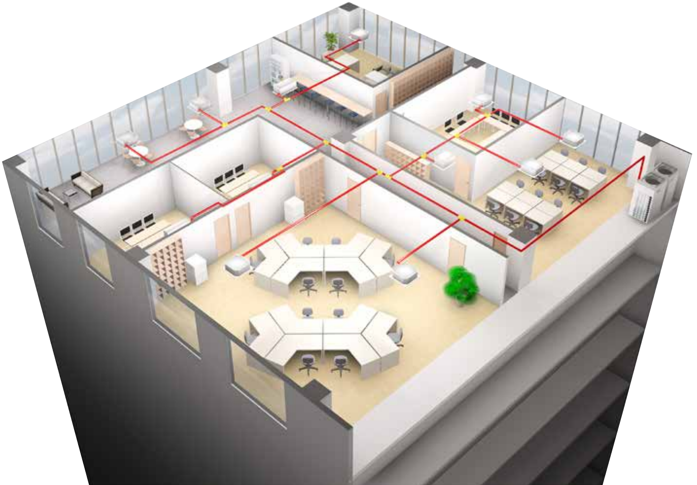
Typical layout of an office suite using Panasonic's VRF Heat Recovery Systems which provides comfort, individual zones and mode control.
